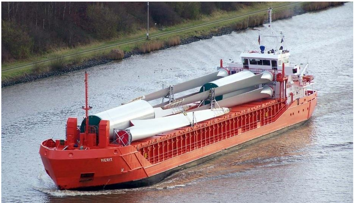
Wind tower sections and wings on deck
