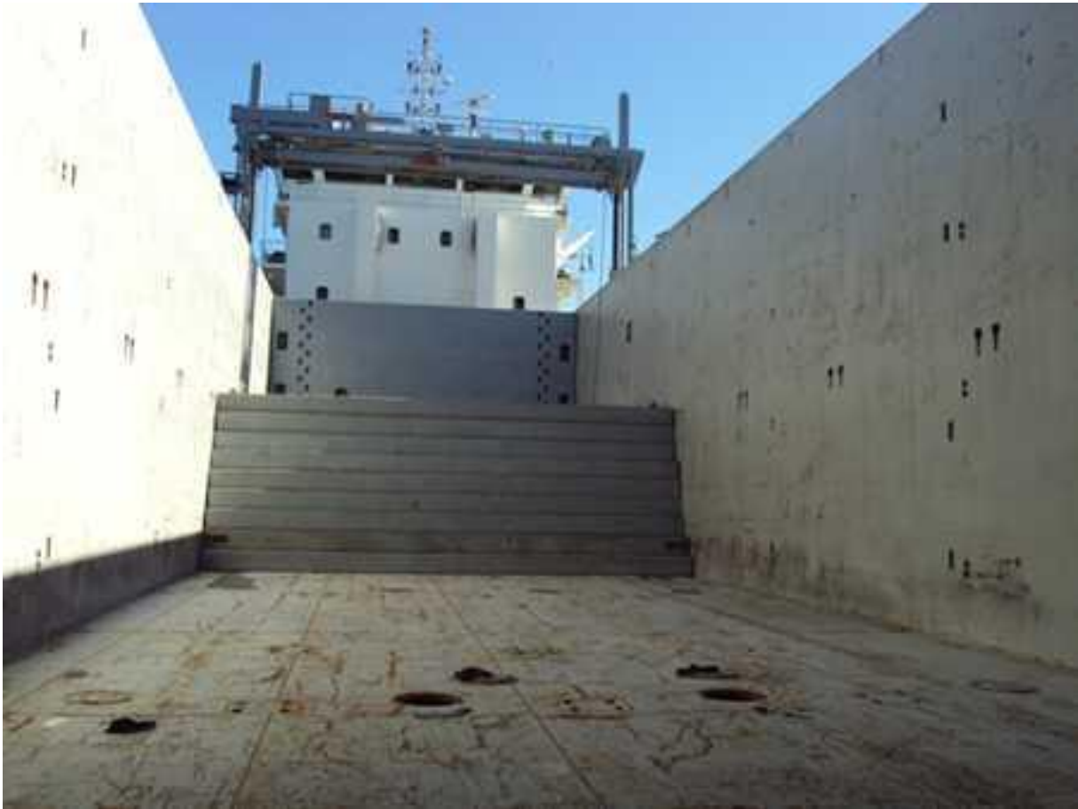
Tweendeck/bulkhead pontoons stowed away aftpart
