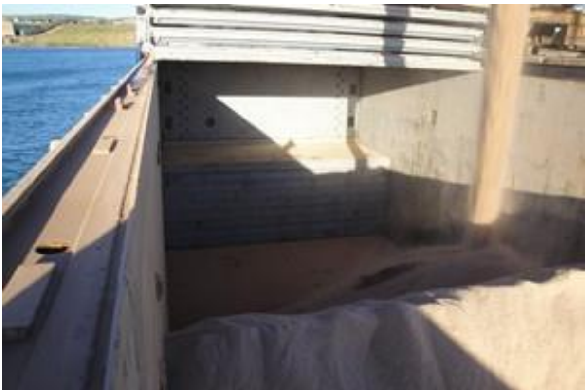
Loading bulk cargo with pontoons stowed away.
